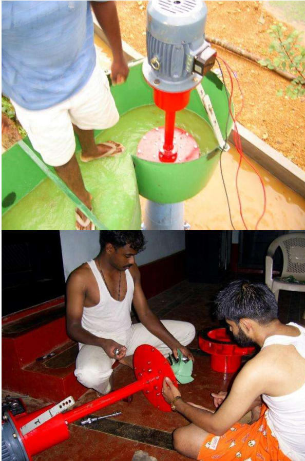
One can see the turbine and the generator in these images. (Image credit: Joy Merwin Monteiro)
